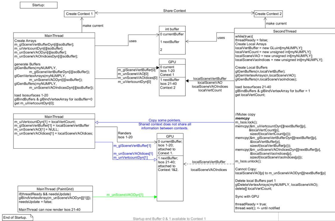
Figure 1: More detailed diagram showing the thread interaction (part 1 of 4). (Created with UMLet 14.2 [www.umlet.com](http://www.umlet.com).)
