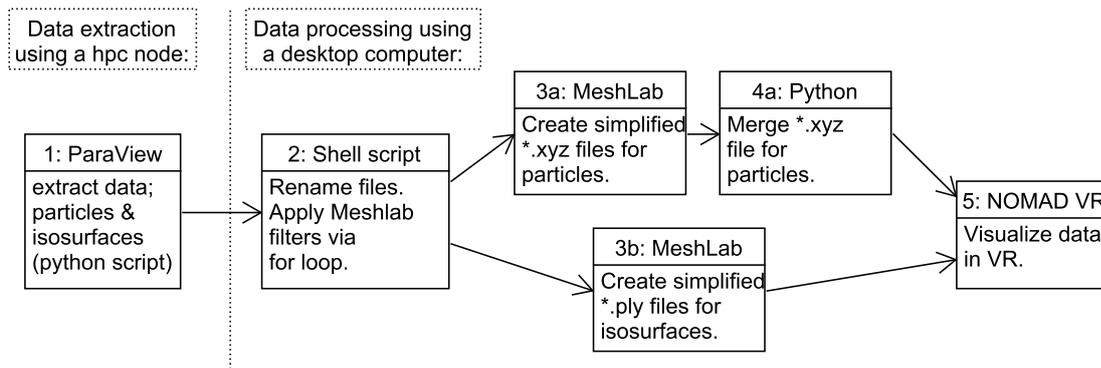
Figure 2.2: Showing the steps to prepare data for NOMAD VR. From left to right: Step 1, 2, 3a & 4a (top branch), 3b (bottom branch) and 5. (Created with UMLet 14.2 [www.umlet.com](http://www.umlet.com).)
