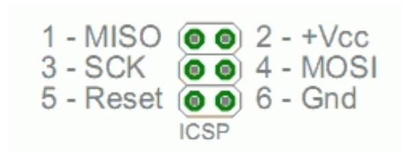
Figure 6.7: ICSP Header (Orientation as in Figure 6.8c) [Ard19]
