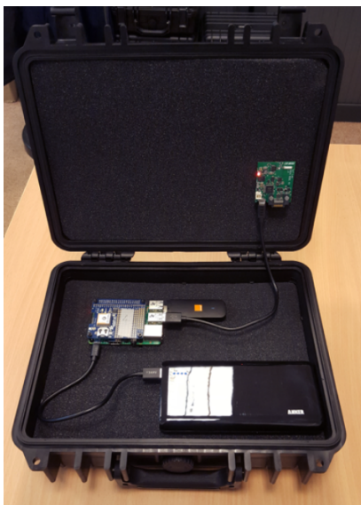
Figure 4.6: Orange SensorLab2 Low-Level Setup [LB17]
